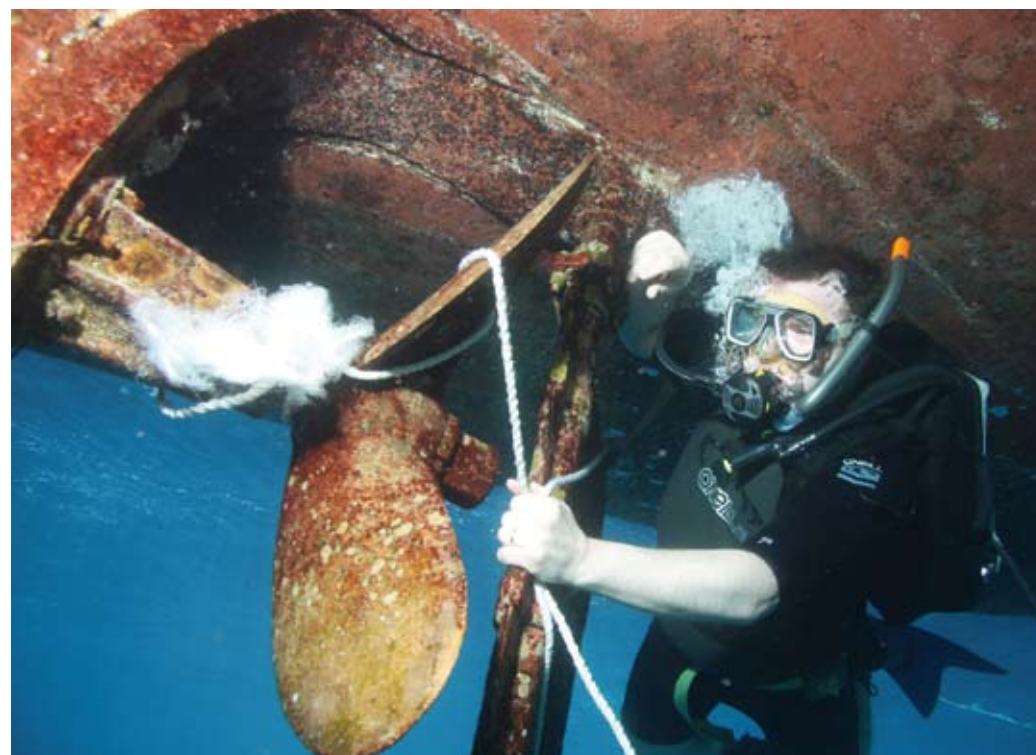
A compelling reason to have this kit aboard: you can free a wrapped propeller
